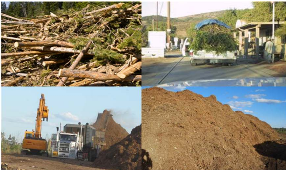
Figure 1. MGW ( top left ); MGW collection ( top right ); portable tub grinder used to shred MGW ( bottom left ); and stockpiled shredded MGW ( bottom right ).
