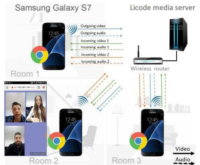
FIGURE 9. Testbed set-up over a LAN connection (User Study 5).
