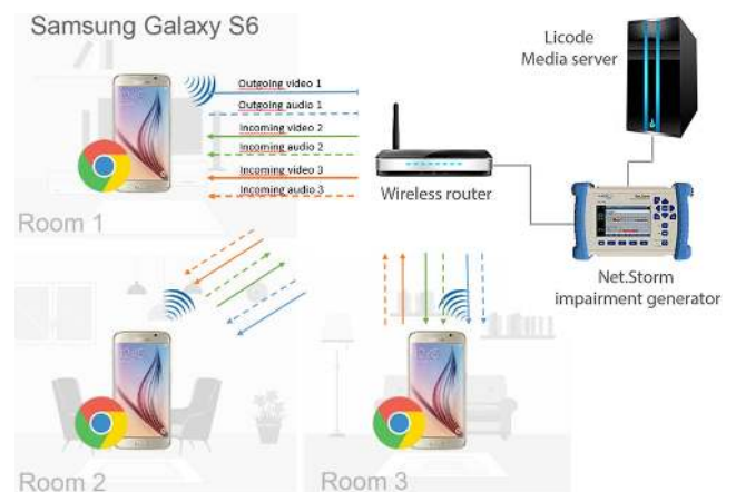
FIGURE 6. Testbed set-up over a LAN connection (User Study 3).
