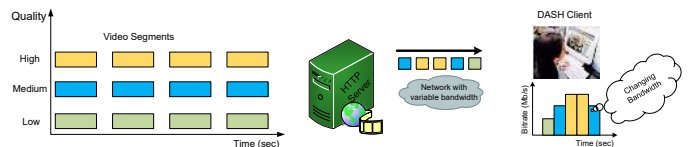
Fig. 9: Dynamic adaptation according to network conditions.
