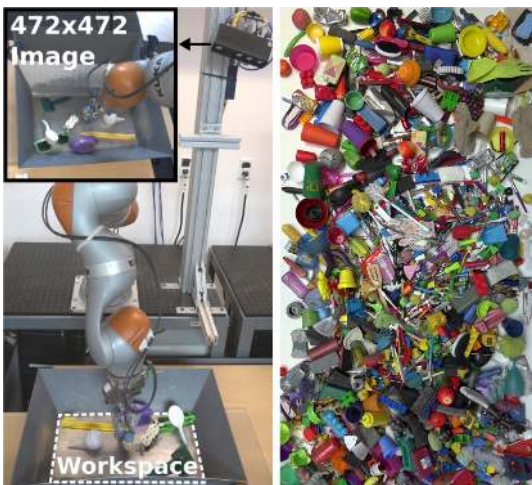
Figure 2: Close-up of a robot cell in our setup (left) and about 1000 visually and physically diverse training objects (right). Each cell (left) consists of a KUKA LBR IIWA arm with a two-finger gripper and an over-the-shoulder RGB camera.
