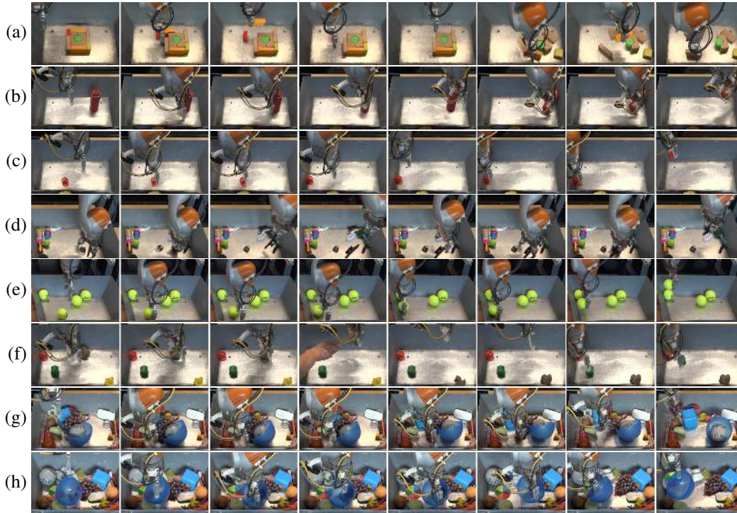
Figure 4: Eight grasps from the QT-Opt policy, illustrating some of the strategies discovered by our method: pregrasp manipulation (a, b), grasp readjustment (c, d), grasping dynamic objects and recovery from perturbations (e, f), and grasping in clutter (g, h). See discussion in the text and Appendix A.
