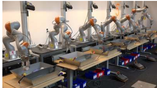
Figure 1: Seven robots are set up to collect grasping episodes with autonomous self-supervision.
