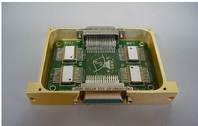
Figure 13. Photograph of a QUaD load resistor board. Each board contains 56 resistors (including eight spares) in four surface-mount packages and services up to 24 channels. The boards themselves are with double-sided 1 oz copper and 8 mil traces. Input and output from the board is via surface-mount 51-way micro-D connectors (Cristek Interconnects Inc., www.cristek.com ). These connectors have long surface-mount leads that take up differential contraction between the fiberglass board and the aluminum mounting structure that provides mechanical support.
