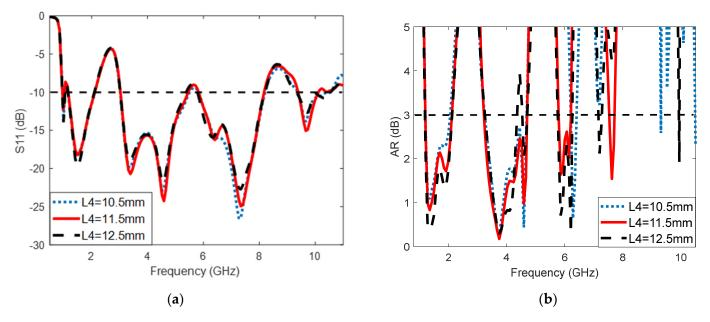
Figure 5. Effect of L4 on antenna performance: (a) S11, (b) AR.
