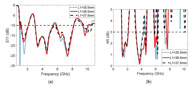
Figure 4. Effect of L1 on antenna performance: (a) S11, (b) AR.
