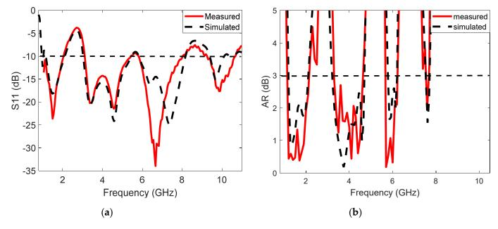
Figure 10. (a) The simulated and measured S11. (b) The simulated and measured AR.
