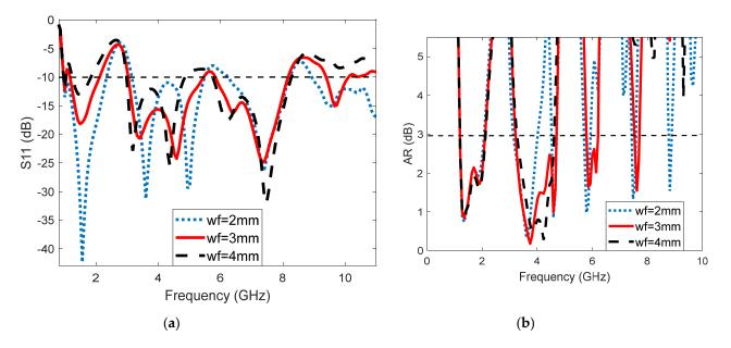
Figure 7. Effect of wf on antenna performance: (a) S11, (b) AR.
