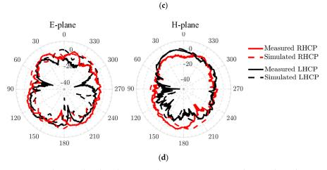
**Figure 11.** The simulated and measured gain patterns, in E plane and H plane, at (**a**) 1.5 GHz, (**b**) 4 GHz, (**c**) 6 GHz, and (**d**) 7.6 GHz.
