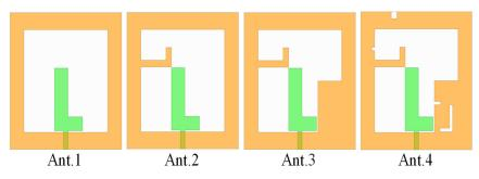
Figure 2. Evolution of the proposed antenna.
