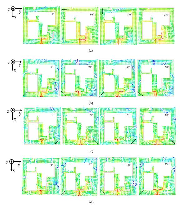
**Figure 8.** Surface current distributions of the proposed antenna at (**a**) 1.5 GHz, (**b**) 4 GHz, (**c**) 6 GHz, and (**d**) 7.6 GHz.
