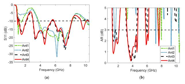
Figure 3. Simulated results for Ant. 1–Ant. 4: (a) S11, (b) AR.
