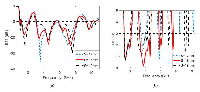
Figure 6. Effect of S on antenna performance: (a) S11, (b) AR.
