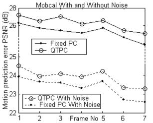
Fig.5. PSNR vs frame no. for the same number of motion vectors for sequence 'Mobcal' with and without noise.
