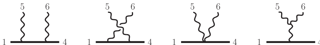
Figure 4. The Compton-amplitude Feynman diagrams. The straight line corresponds to the spinning particle. The wiggly lines correspond to gravitons.
