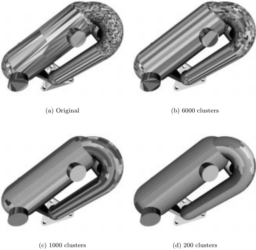
Figure 8.4: Sample clusters on the heat exchanger.
