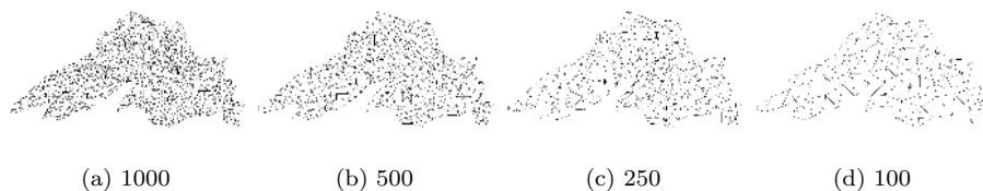
Fig. 11. A planar mesh of the interior of Lake Superior is reduced from an initial size of 2894 vertices down to 100.
