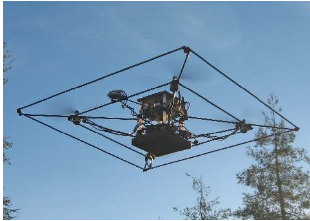
Figure 1. Autonomous hover at a waypoint by a quadrotor helicopter from the Stanford Testbed of Autonomous Rotorcraft for Multi-Agent Control (STARMAC).
