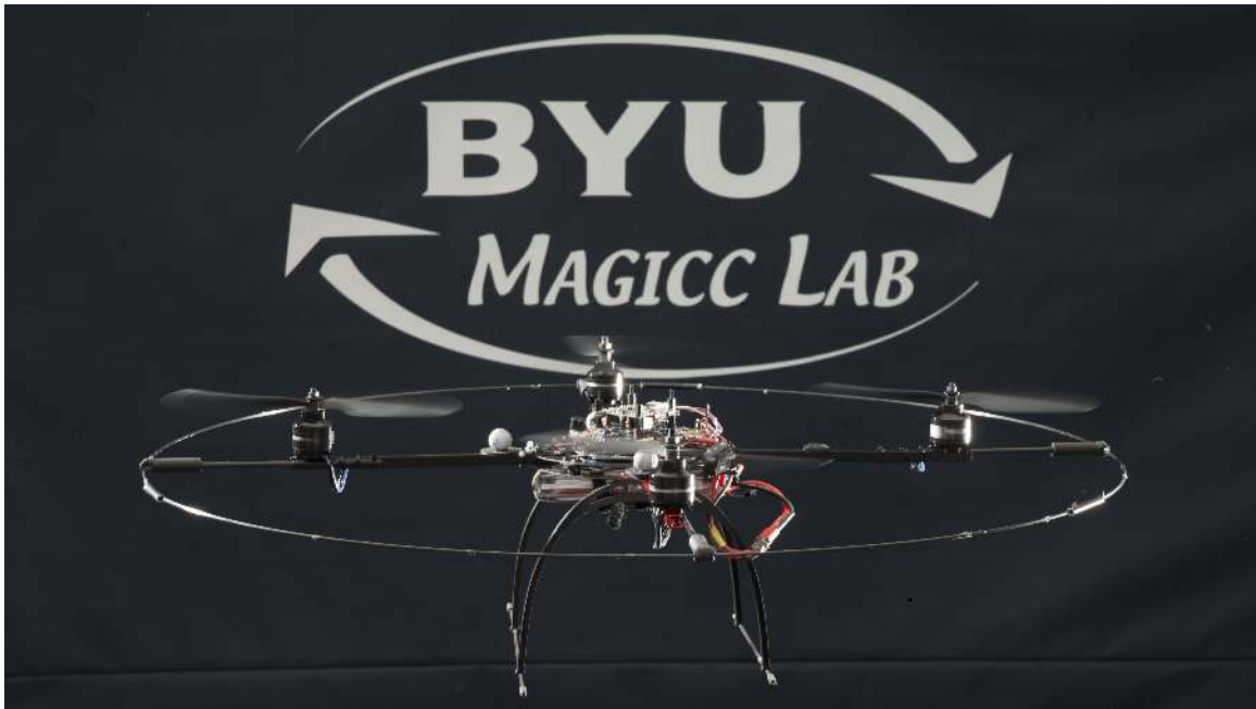
Figure 5: Hovering Quadrotor. A quadrotor from MikroKopter that was used in the experiments. The vehicle is hovering using the measurements from the motion-capture system. ©Jaren Wilkey, BYU Photo
