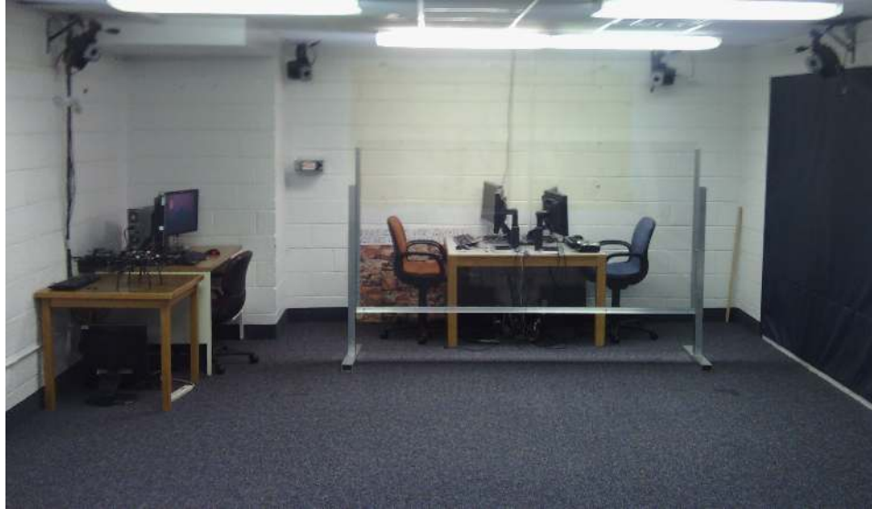
Figure 6: Motion-capture Environment. The motion-capture environment where all the testing was conducted for this article uses a motion-capture system from Motion Analysis. The system provides 6DoF pose information at 200 Hz with sub-degree and sub-millimeter accuracy.
