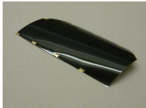
Figure 1. Typical figure of bare IMM-3J solar cells after completion of the fabrication process.
