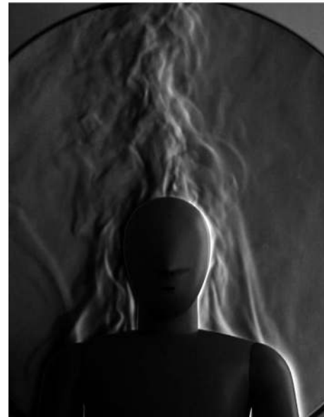
FIGURE 4 Example vertical-knife-edge schlieren image from the 500-image ensemble used for thermal plume analysis
