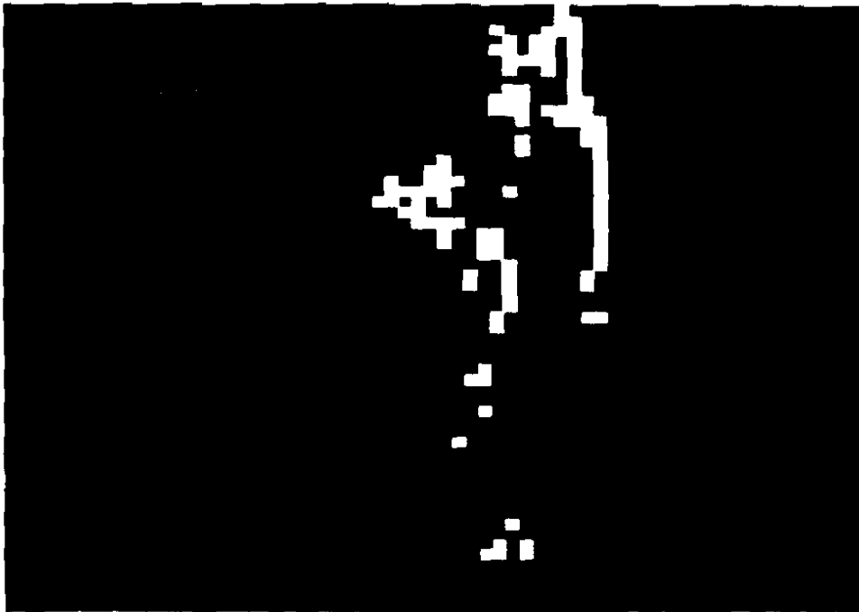
Figure 7: Detection of a walking figure in a moving scene by a movement detector based on constraint ray matching. The camera motion is a combination of rotation and translation whose net effect is to provide impart upward apparent motion (at velocities which depend on distance) to objects in the scene. The walking figure is detected as inconsistent with a rigid interpretation of the motion. The system operates in real time (10 frames/sec).
