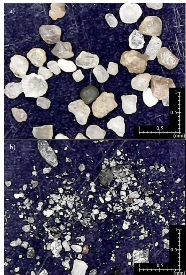
Fig. 2. Microscopy images of a) Ham River sand and b) Øysand particles.
