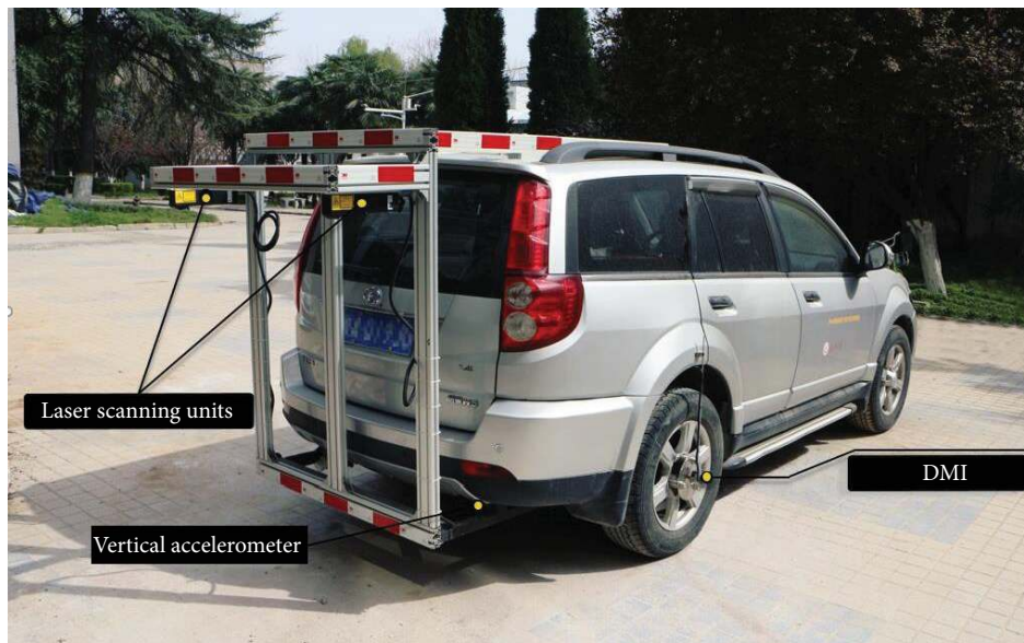
FIGURE 2: Configuration of the laser scanning vehicular system (LSVS).
