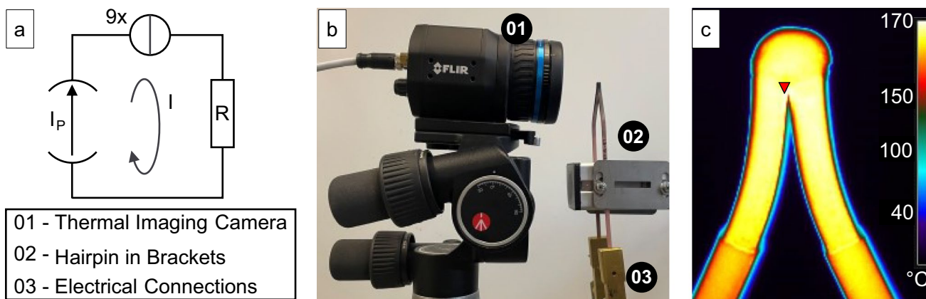
Fig. 7 Thermography of electrically stressed hairpin contacts; a circuit diagram; b experimental setup; c output image of the camera
