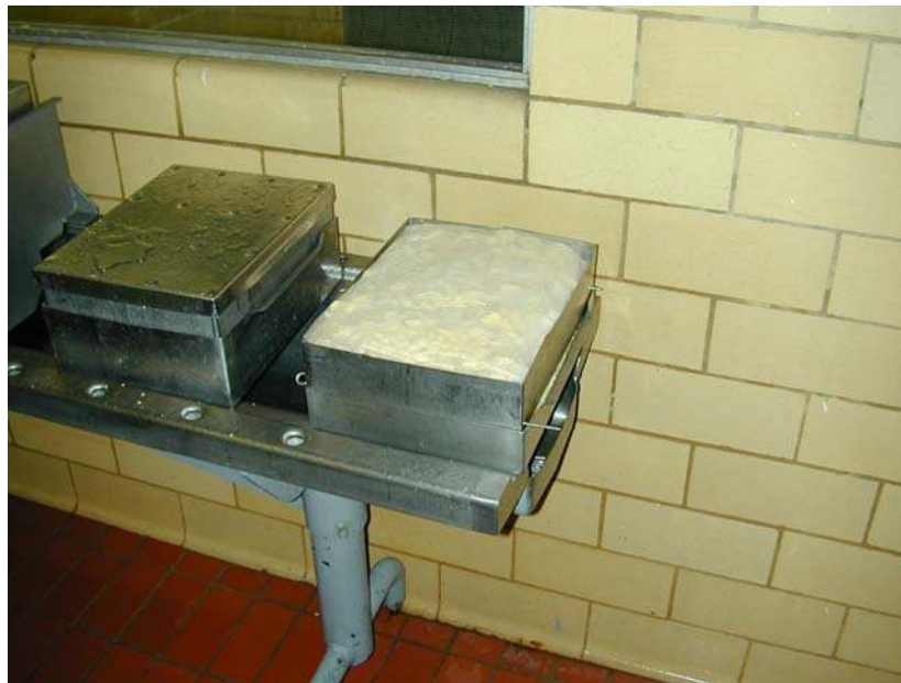
Figure 3.24: 40 pound hoops with cheesecloth wrapping the salted curd.
