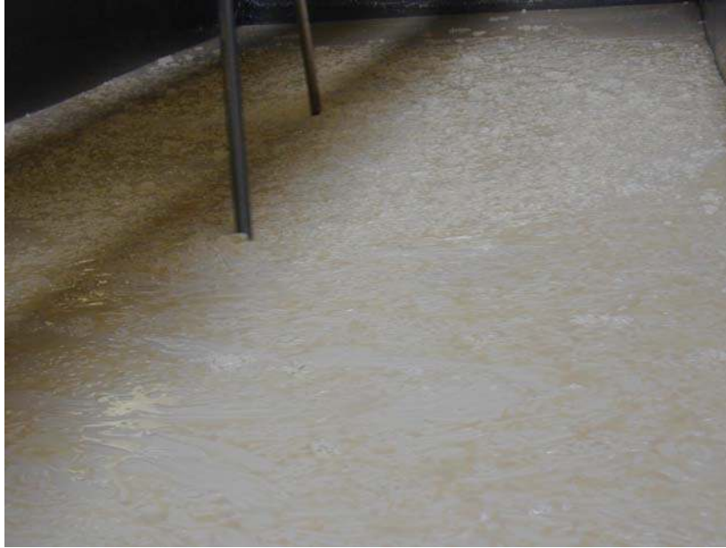
Figure 3.14: Cooking the curd with agitation and increasing the temperature.
