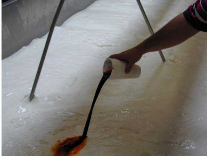
Figure 3.5: Adding color to heated milk after starter culture was added.
