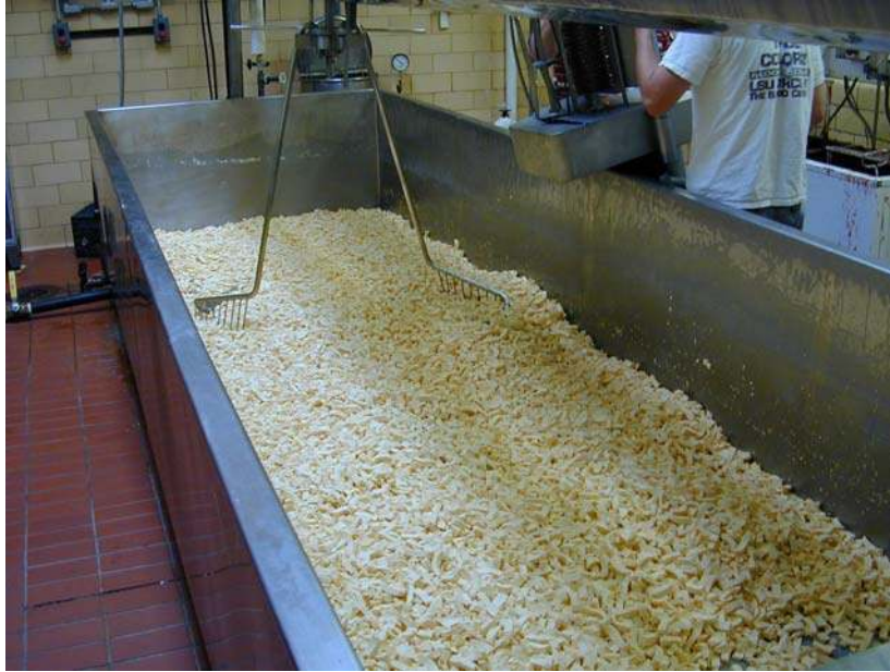
Figure 3.23: Mixing salt with the milled curd which lasted approximately 30 minutes.
