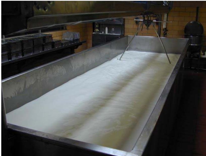
Figure 3.2: Stirring milk in the vat while being heated up before adding culture.
