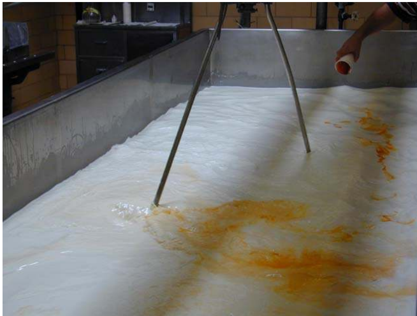
Figure 3.6: Color added to heated milk while stirring.
