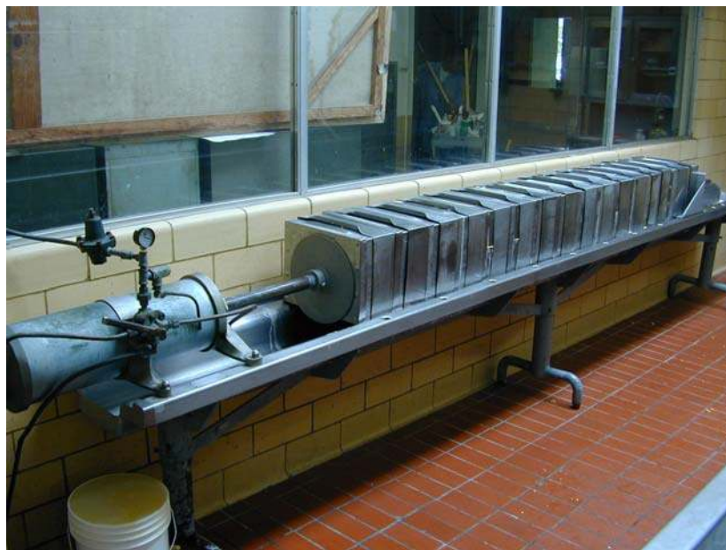
Figure 3.25: Hoops filled with the curd pressed under 50 psi pressure overnight.
