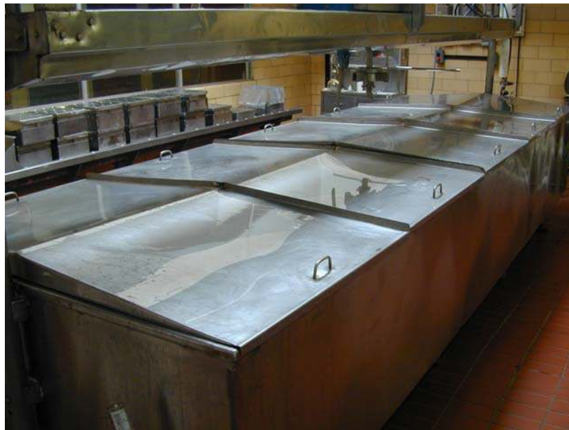
Figure 3.9: Renneting taking place in the vat while the temperature was still 88°F.
