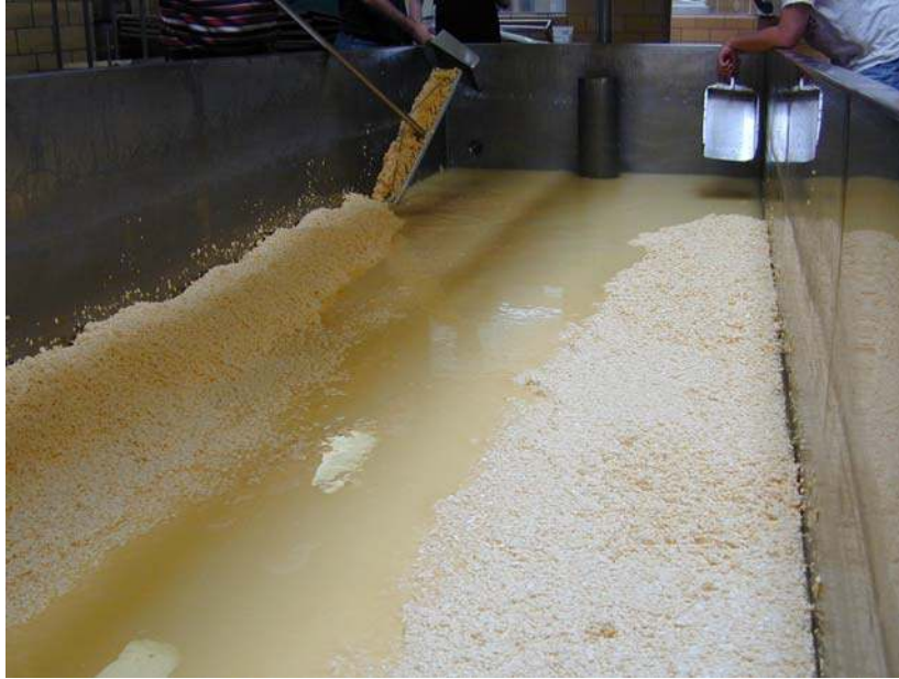
Figure 3.16: Draining of whey protein, while keeping the curd inside vat.
