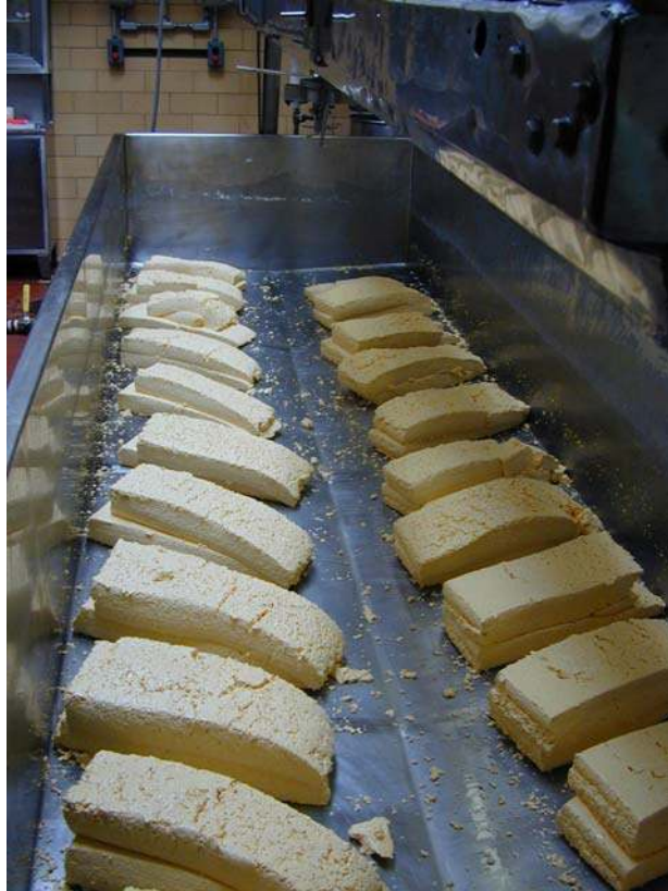
Figure 3.20: Two loaves of curd stacked to help release of whey protein in vat.
