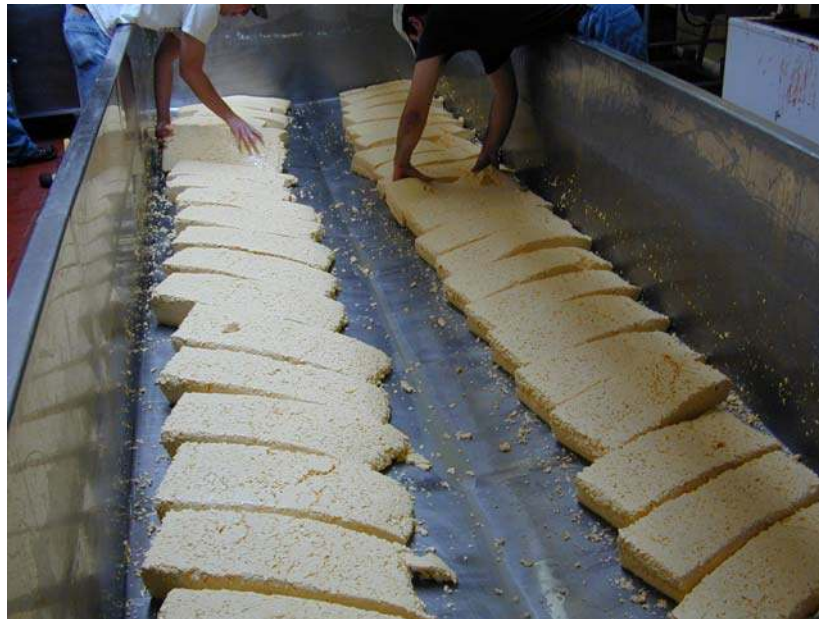
Figure 3.19: Flipping loaves over to help drain whey protein out of the curd.
