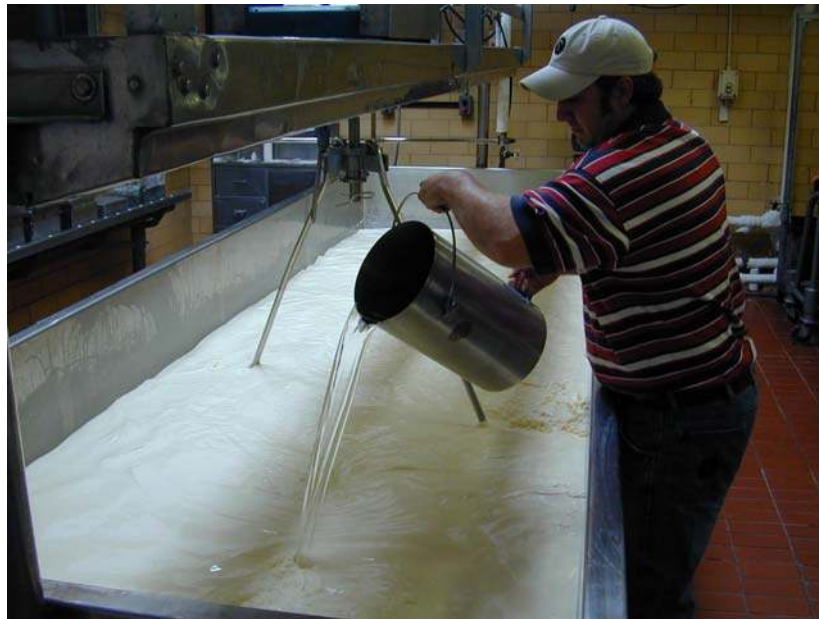
Figure 3.8: Adding the rennet into the milk after the culture, color and \text{CaCl}_2 were added.
