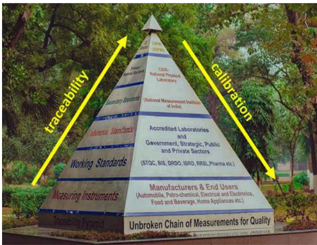
Fig. 4 Photograph of a 3-dimensional model of metrology traceability pyramid at the NPLI campus showing the unbroken chain of measurements traceable to the SI units and the responsible organizations in India for dissemination of metrology traceability to manufacturers and end users (The pyramid was installed in 2016 based on the concepts of Dr. D. K. Aswal and Dr. V.N. Ojha)
