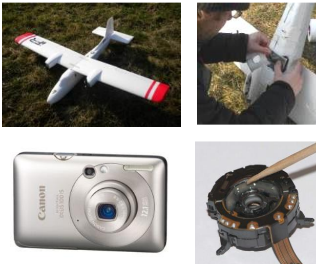
Figure 1: Platform Twinstar Multiplex (top) and Canon Ixus 100 camera with fixed lens element (bottom).
