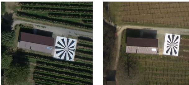
Figure 4: Image sections depicting the Siemens star for Ricoh flown August, 23 rd (left) and Canon flown March, 23 rd (right)
