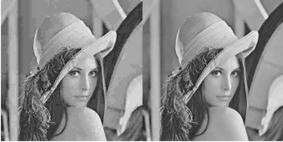
Fig 1. The blocking artifacts are obviously shown in JPEG image. The “Lena” image was compressed around 20:1 by JPEG (left) and JJ2000 (right).
