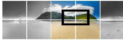
Fig. 6. In tiled VR streaming, the 360° video is divided into spatial regions. Only tiles belonging to the viewport are streamed at the highest quality, to save bandwidth.
