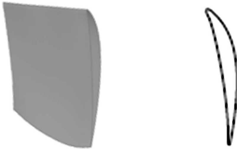
Figure 3.4: Schematic picture of a vane (left) and the corresponding cross-section (right).
