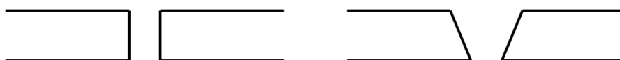
Figure 2.10: An illustration of weld cross sections for different joint designs: squared butt joint (left) and a grooved joint (right).
