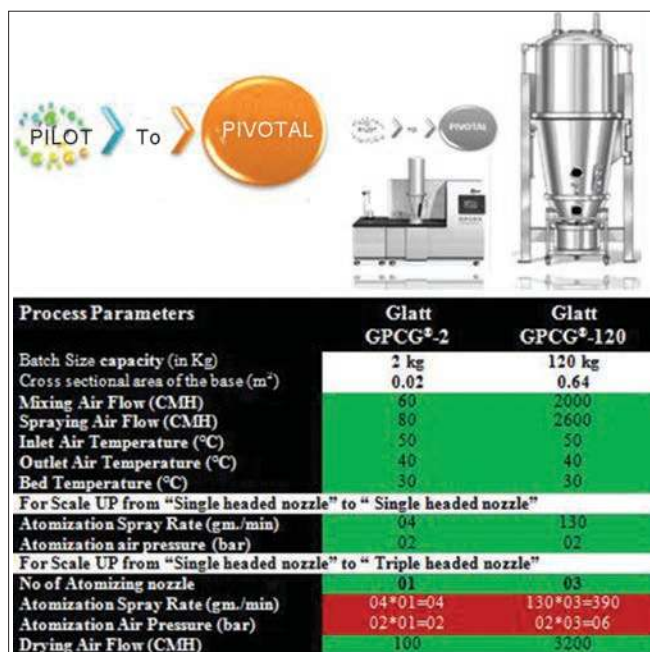
Figure 8: Controlled FBP Parameters from small lab scale to large production scale
