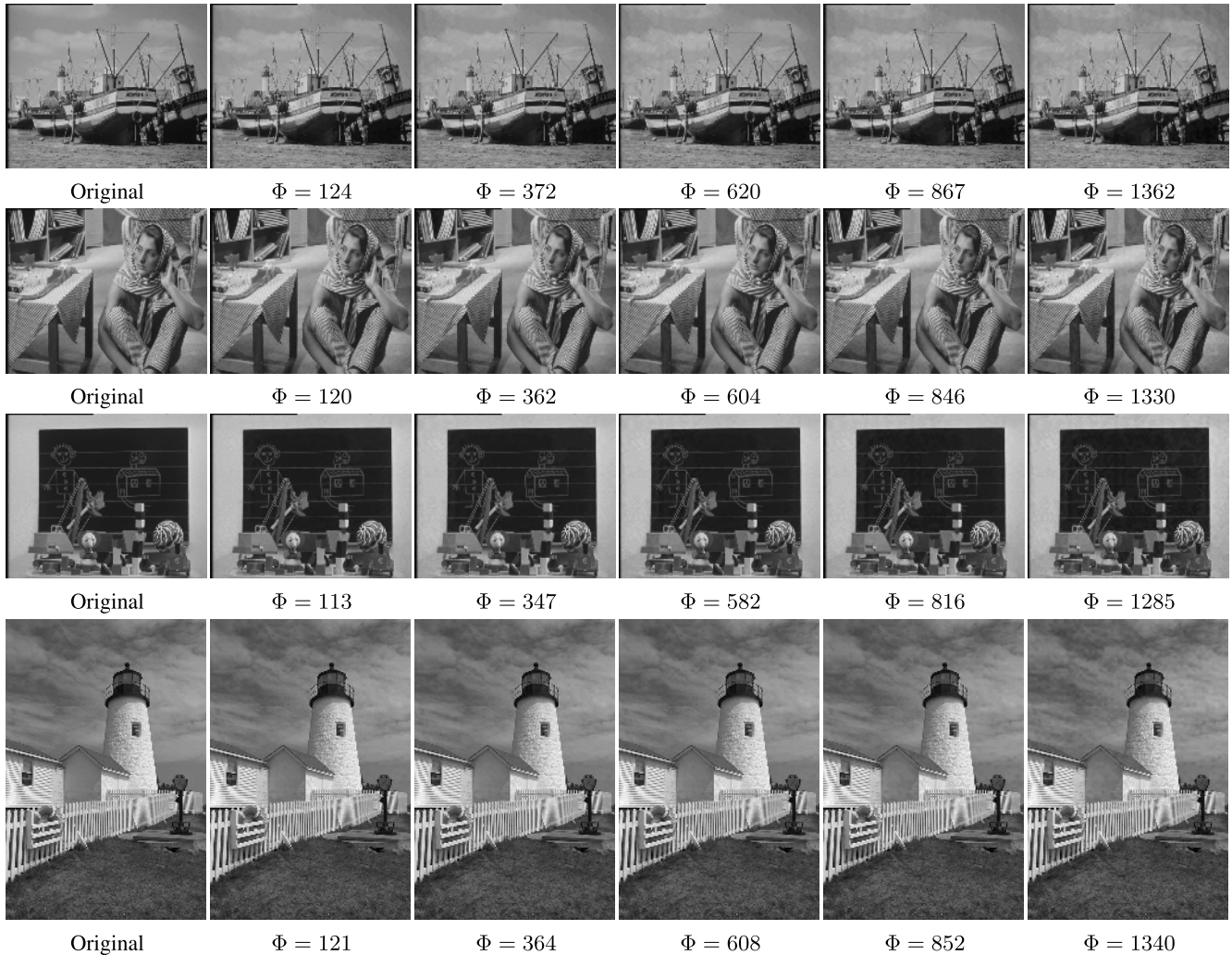
Fig. 12. Visual representation of watermarked images at various rate points for Row 1) Boat 2) Barbara 3) Blackboard and 4) Light House.
