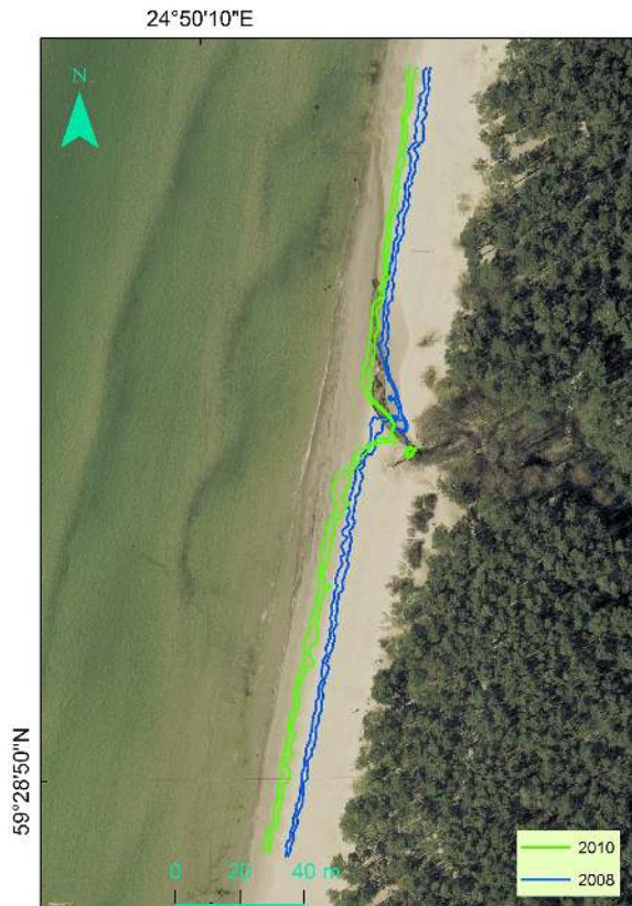
Fig. 4. Changes in the position of the waterline (0.5 m and 0.6 m isolines) from 2008 to 2010.
