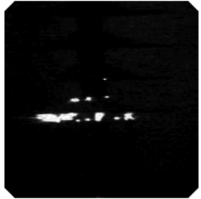
(c) Corona from water drops on weathershed at 50 kV (0.75 p.u)
