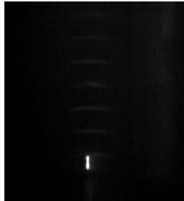
(e) Corona in the shank between hardware and the first shed at 60 kV (0.9 p.u) under wet conditions
