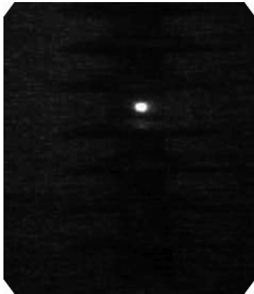
(d) Corona from water drops in the interface of shed and shank at 40 kV (0.60 p.u)
