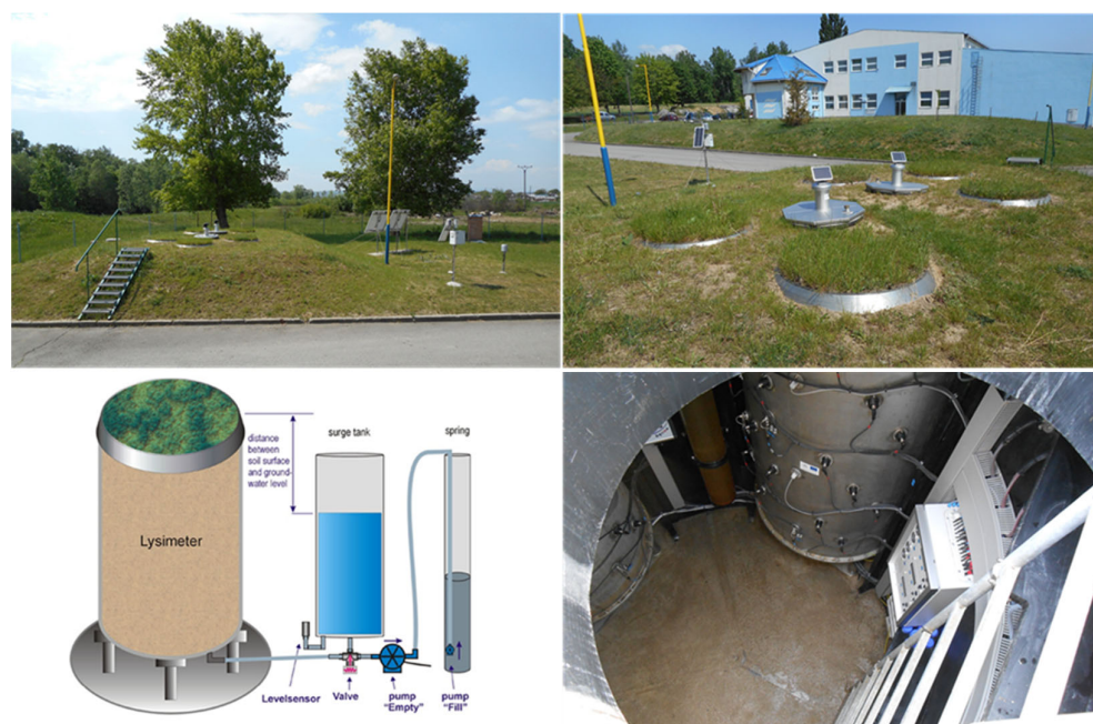
Figure 2. Lysimetric station in the Petrovce nad Laborcom with lysimeter function design.
