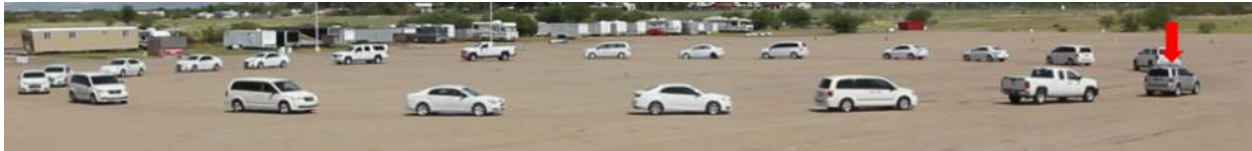
(c) Alignment of vehicles 328 seconds into Experiment A when the CAT Vehicle is actively dampening the wave.
