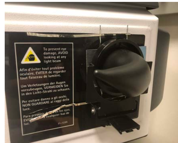
Test cell and light trap on the spectrophotometer.
