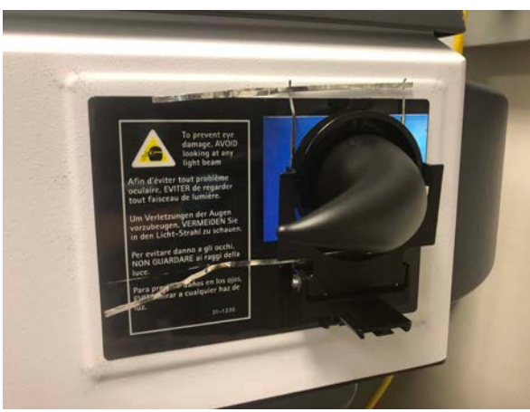
Test cell and light trap on the spectrophotometer.
