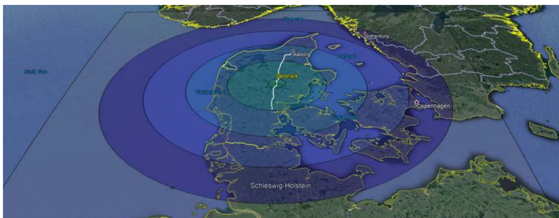
Fig. 10 Impact PDF for a flyaway event for the aircraft fully fueled at the start of the flight. The event location is WP 39. There is a very small yellow zone in the middle of the concentric contour lines, which is the vertical flyaway zone. But it is too small to be visible in this view. The
