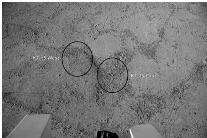
Fig. 9. Field of view of the two downlooking KT15.85 IIP radiometers, on the gravel plain north of Gobabeb LST validation station (KT-15 West and KT-15 East). The ellipses cover about 13 m 2 (horizontal diameter about 3.7 m).
