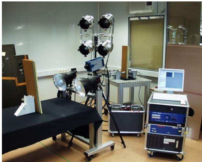
Figure 5.2: Thermography set-up of the Edevis company.
