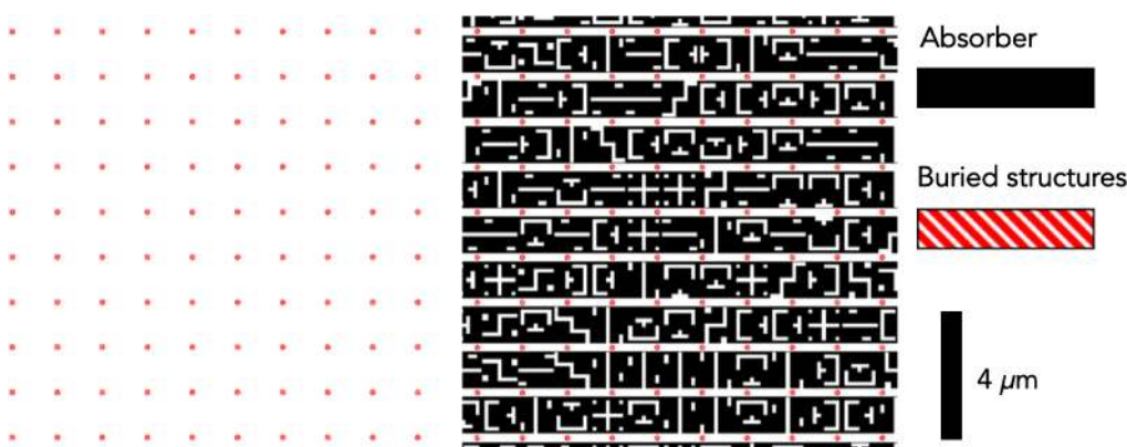
Fig. 6 Detail of the sample layout including buried carbon structures and HSQ absorber pattern. The carbon structures consist of 800 nm 1:1 lines and dots with 200 nm diameter and 2 \mu\text{m} pitch. The absorber pattern consists of a logic-like pattern with 200-nm CD.
