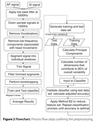
**Figure 2 Flowchart.** Process flow steps outlining the preprocessing feature extraction and selection and classification techniques, as described in Methods.
