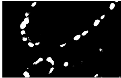
(b) CCD Sensor - After Med. Filtering and Thresholding
