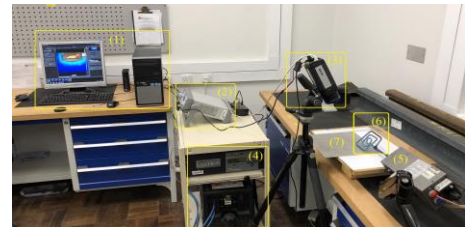
Fig.5. Experimental setup: (1) computer with software, (2) signal generator, (3) IR camera, (4) EasyHeat induction heating system, (5) work head, (6) coil, (7) sample under test.
