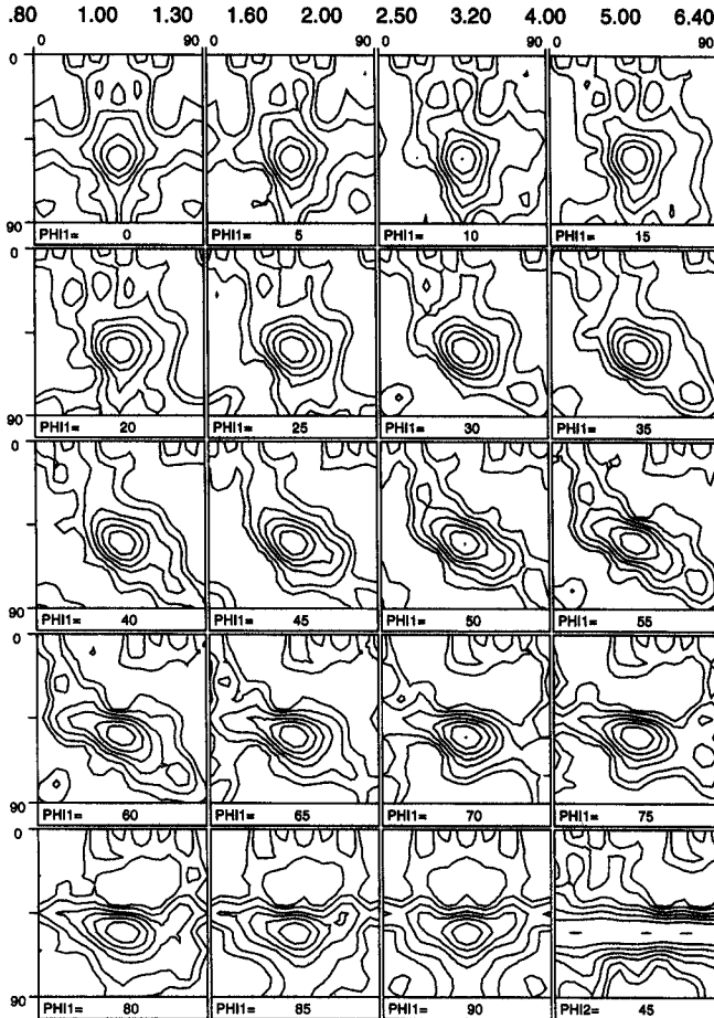
FIGURE 17 ODF of another hot rolled steel, used as initial texture for a second case study.
