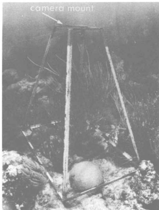
Figure 4. Quadrat frame and camera mount used in Belt quadrat transects in place on sea floor, North Rock.
