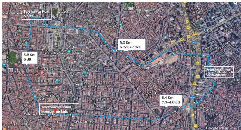
Figure 1: The Madrid SDN QKD Network layout installed in Telefónica of Spain production network. The distances and losses between the Points of Presence used are given in the white boxes. The additional losses in some of the links correspond to additional fibre (spool) used to artificially increase the distances in some experiments. Note that losses are much higher than the expected because of the distance, since additional connectors, bending of the fiber and crossing of intermediate PoPs (not shown) have an important impact.
