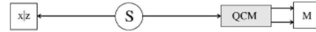
FIG. 1. Setup devised by Herbert to achieve signaling. A source S produces pairs of qubits in a maximally entangled state; on the left, Alice measures either \sigma_x or \sigma_z . On the right, Bob applies a perfect quantum cloning machine (QCM) and then measures the two clones (the measurement M may be individual or collective).
