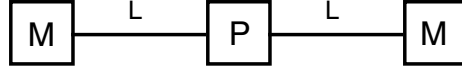
FIG. 1: Schematic of long-distance quantum communication system: P = ultrabright narrowband source of polarization-entangled photon pairs; L = L km of standard telecommunications fiber; M = trapped-atom quantum memory.
