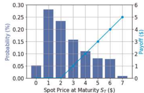
Fig. 6 Payoff function European Call option. Probability distribution of the spot price at maturity S_T and the corresponding payoff function for a European Call option. The distribution has been learned with a randomly initialized qGAN run on the IBM Q Boeblingen chip.
