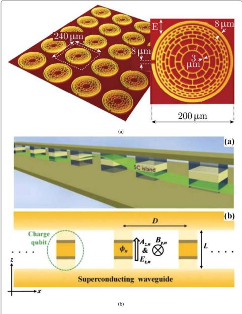
**Figure 2 Superconducting quantum metamaterials. (a)** A 2D superconducting quantum metamaterial [24] (Figure 3 of [24]). **(b)** A realization of a 1D superconducting quantum metamaterial: charge qubits in a transmission line [31].
