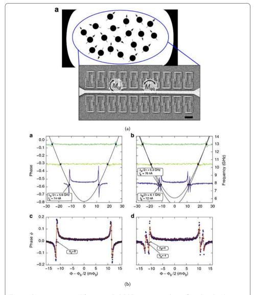
**Figure 5 Quantum metamaterial prototype [36]. (a)** Twenty superconducting flux qubits placed in a resonator. The signal wavelength is of the order of the resonator length (23 mm) and greatly exceeds the qubit size (approx.  $2 \times 6 \mu m$ ). The ensemble average level spacing and persistent current in the qubits are 5.6 GHz and 74 nA respectively. **(b)** The QMM in the resonant regime. Three distinct qubit ensembles are seen.
