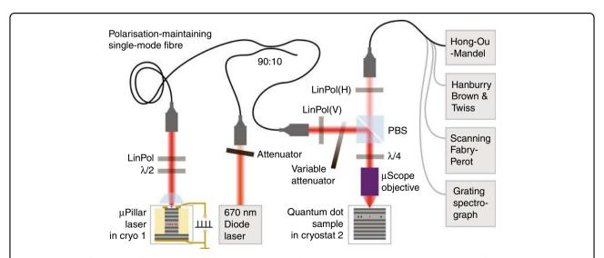
**Fig. 1 Schematic illustration of the experimental concept.** Emission of the electrically driven microlaser in cryostat 1 is fiber-coupled to resonantly excite a single QD in cryostat 2. Applying either CW or pulsed excitation, dressing of the two-level system or triggered emission of single photons can be observed and verified by high-resolution spectroscopy and single-photon counting
