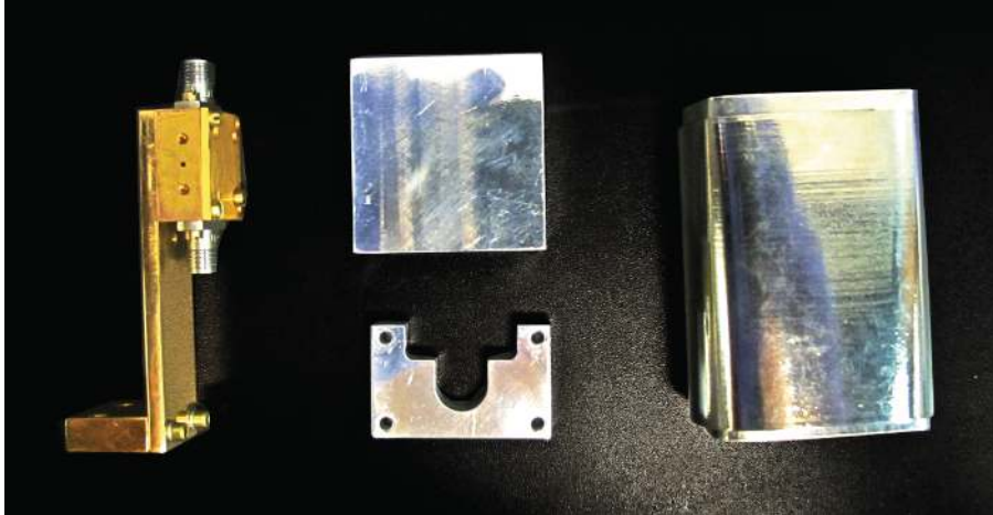
Figure 3.3: Additional aluminum shield (center) fits over both the sample package and cold finger (left), and includes a hole in the top for accessing the output SMA connector. The aluminum cap is then bolted to the bottom, and the whole finger is covered with the mu-metal and Metglas shield (right).
