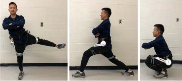
Fig. 4. Demonstration of the range of motion of the robot. The hip exoskeleton is designed with a wide range of motion to support the wearer to perform various activities.
