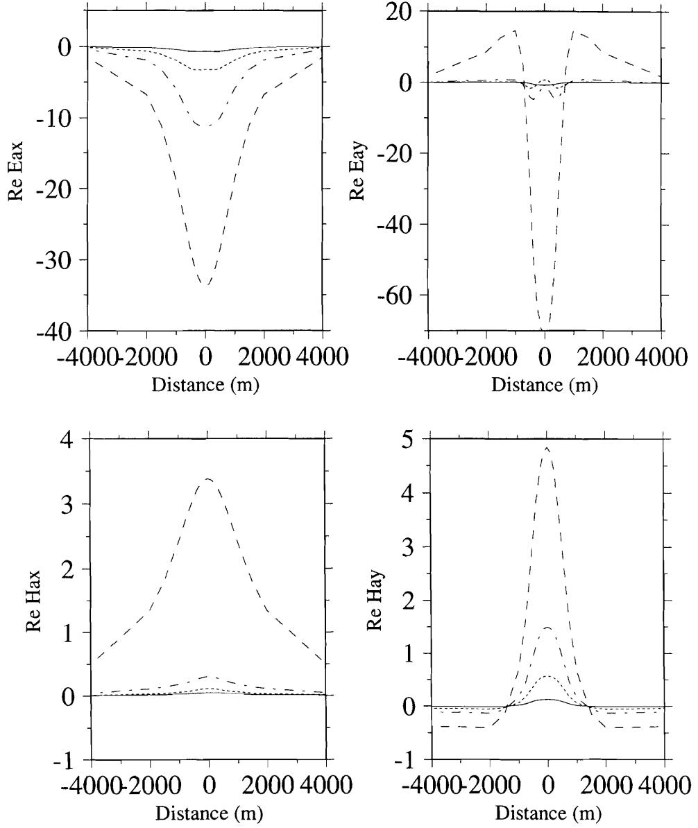
**Figure 7.** Numerical comparison of full IE solution (solid line), the modified Born approximations of the first order (dashed line), the third order (dash-dotted line), and the fifth order (dotted line) computed for model 3 (Figure 6) at frequency 1 Hz. Calculations are done for receivers located along the Y axes on the surface.
