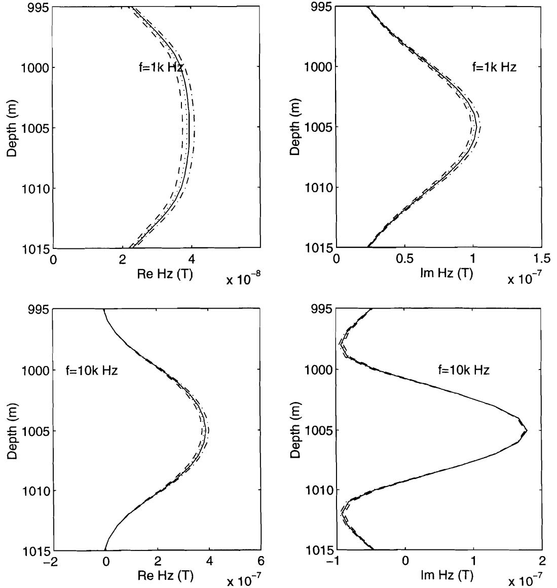
**Figure 5.** Numerical comparison of full IE solution (solid line), QL approximation (dashed line), second-order QL approximation (dash-dotted line), and third-order QL approximation (dotted line) computed for model 2 (Figure 1b) at frequencies 1 and 10 kHz. Calculations are done for receivers moved along the borehole.
