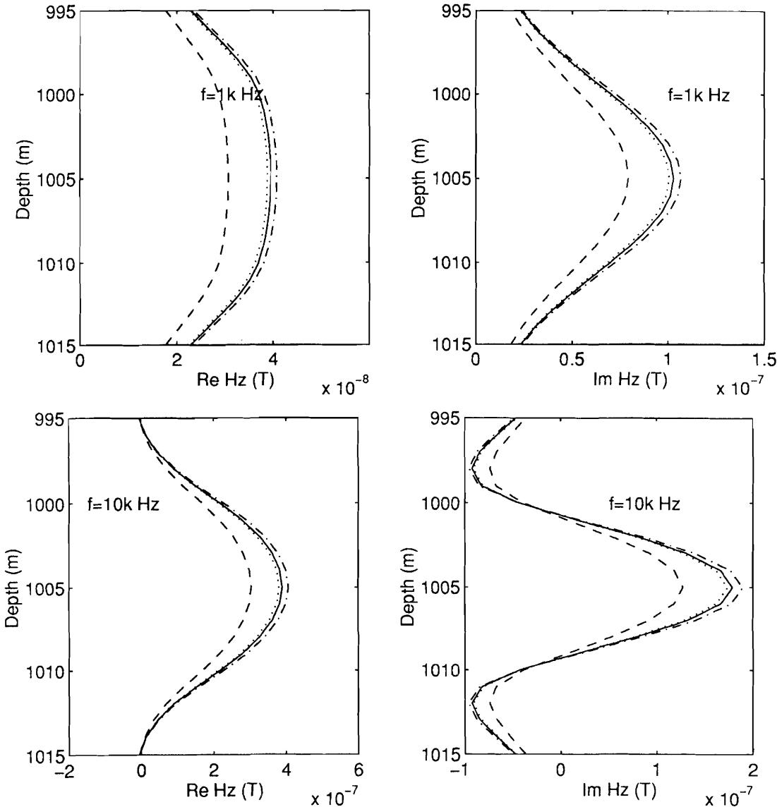
**Figure 4.** Numerical comparison of full IE solution (solid line), Born approximation (dashed line), second-order modified Born approximation (dash-dotted line), and third-order modified Born approximation (dotted line) computed for model 2 (Figure 1b) at frequencies 1 and 10 kHz. Calculations are done for receivers moved along the borehole.
