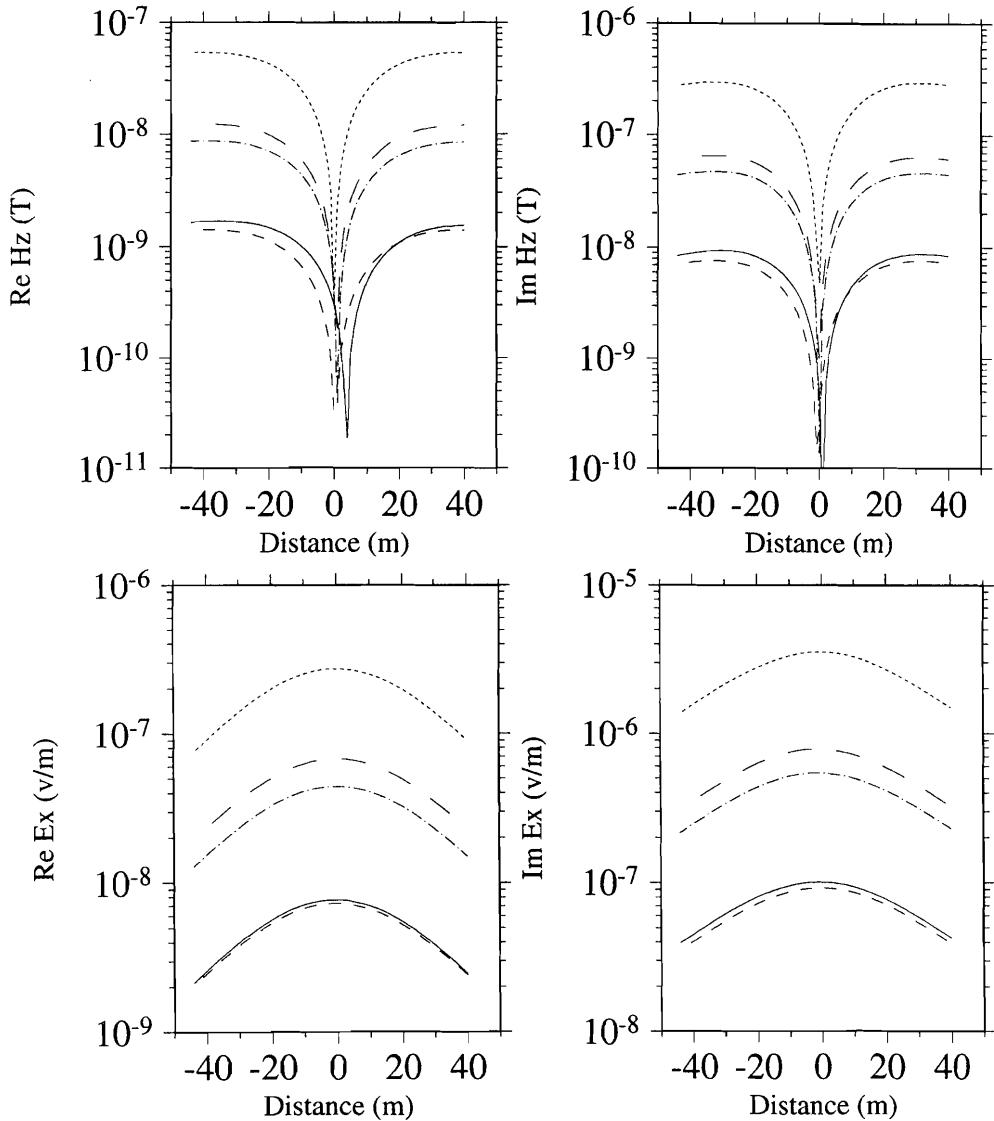
**Figure 2.** Numerical comparison of full integral equation (IE) solution (solid line), QL approximation (short-dashed line), Born approximation (dotted line), second-order modified Born approximation (long-dashed line), and third-order modified Born approximation (dash-dotted line) computed for model 1 (Figure 1a) at frequency 1000 Hz. Calculations are done for receivers located along the  $Y$  axes on the surface.
