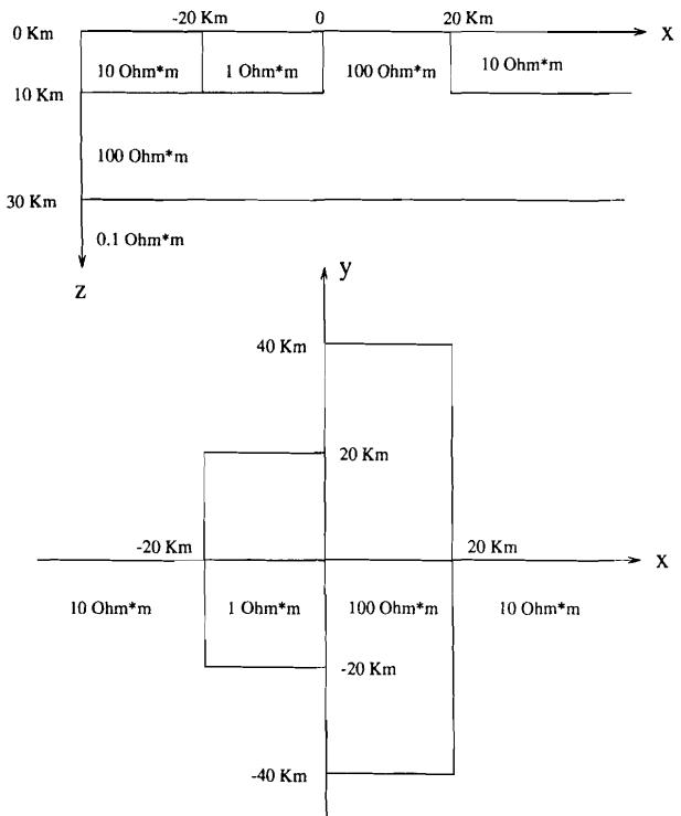
**Figure 10.** Three-dimensional geoelectric model containing one conductive body and one resistive body in a three-layer background resistivity cross section with resistivities 10, 100, and 0.1 Ohm-m and with a plane wave excitation (model 4).
