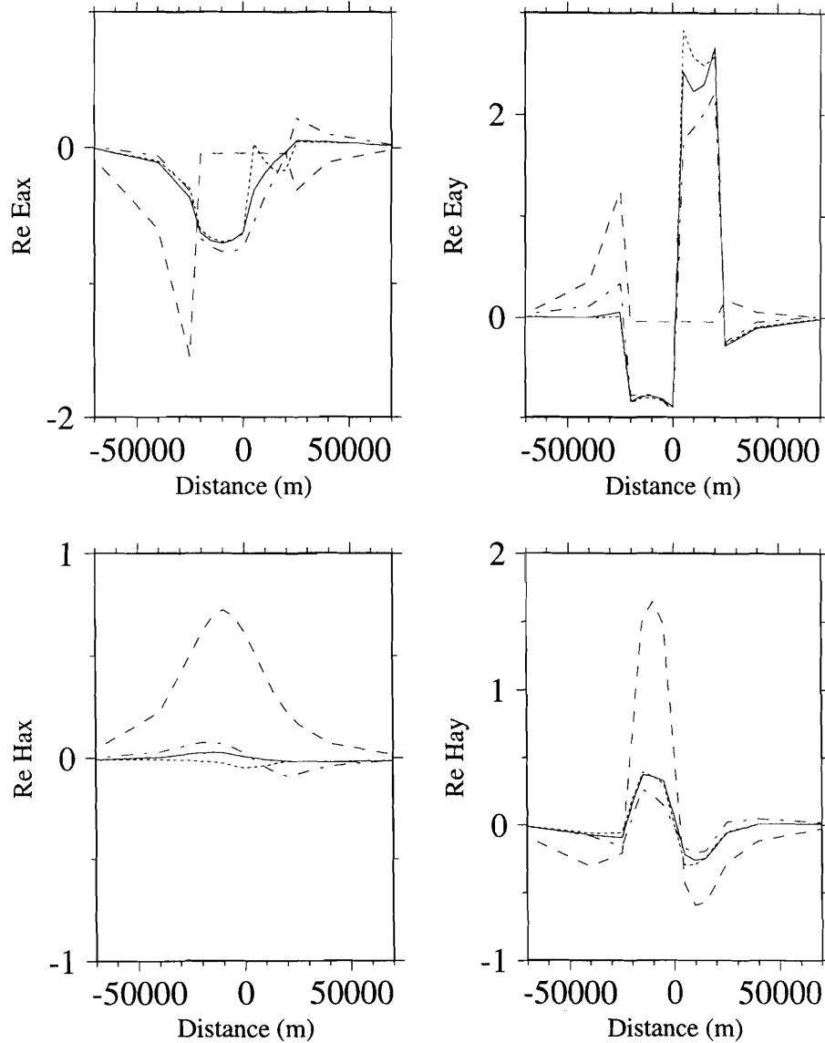
**Figure 11.** Numerical comparison of full IE solution (solid line), the modified Born approximations of the first order (dashed line), the third order (dash-dotted line), and the fifth order (dotted line) computed for model 4 (Figure 10) at frequency 0.01 Hz. Calculations are done for receivers located along the  $Y$  axes on the surface.
