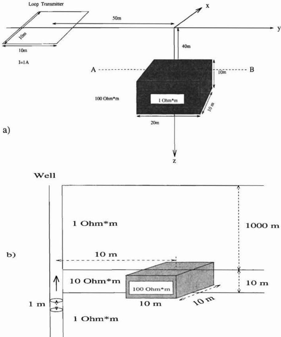
**Figure 1.** (a) Three-dimensional (3-D) model of rectangular conductive structure in a homogeneous half space, excited by a rectangular loop, and (b) 3-D borehole model of cube resistive structure in a three-layer background model, excited by a vertical magnetic dipole.
