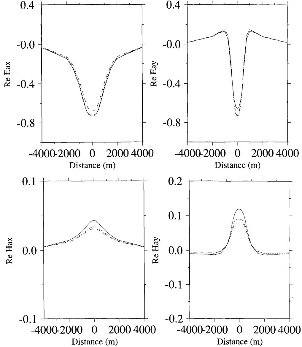
**Figure 9.** Numerical comparison of full IE solution (solid line), the QL approximations of the first order (dashed line), and the third order (dotted line), computed for model 3 (Figure 6) at frequency 1 Hz. Calculations are done for receivers located along the Y axes on the surface.
