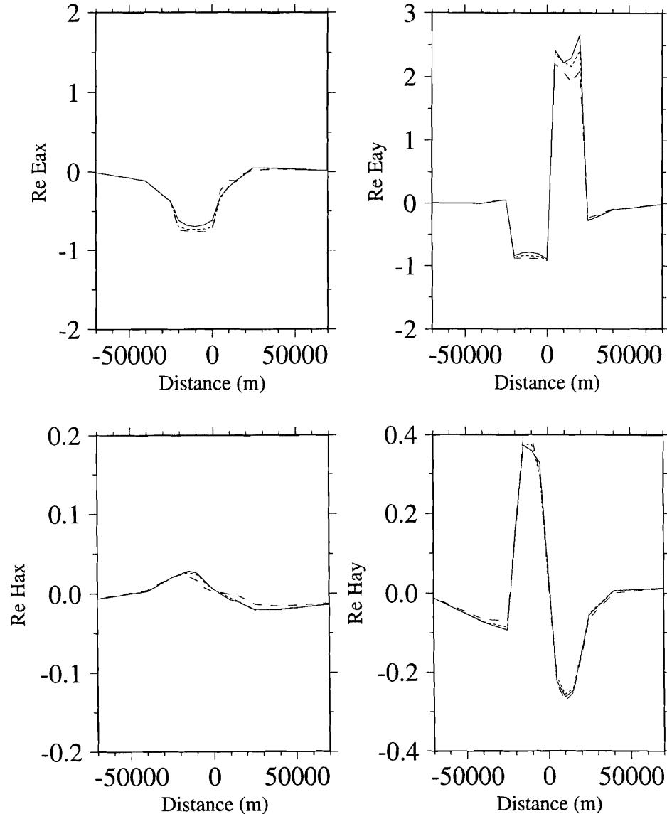
**Figure 13.** Numerical comparison of full IE solution (solid line), the QL approximations of the first order (dashed line), and the third order (dotted line), computed for model 4 (Figure 10) at frequency 0.01 Hz. Calculations are done for receivers located along the  $Y$  axes on the surface.
