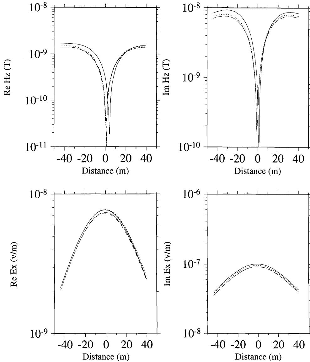
**Figure 3.** Numerical comparison of full IE solution (solid line), QL approximation (dashed line), second-order QL approximation (dash-dotted line), and third-order QL approximation (dotted line) computed for model 1 (Figure 1a) at frequency 1000 Hz. Calculations are done for receivers located along the  $Y$  axes on the surface.
