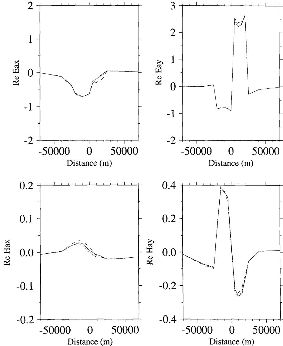
**Figure 12.** Numerical comparison of full IE solution (solid line), the modified Born approximations of the seventh order (dashed line), and the ninth order (dotted line) computed for model 4 (Figure 10) at frequency 0.01 Hz. Calculations are done for receivers located along the  $Y$  axes on the surface.
