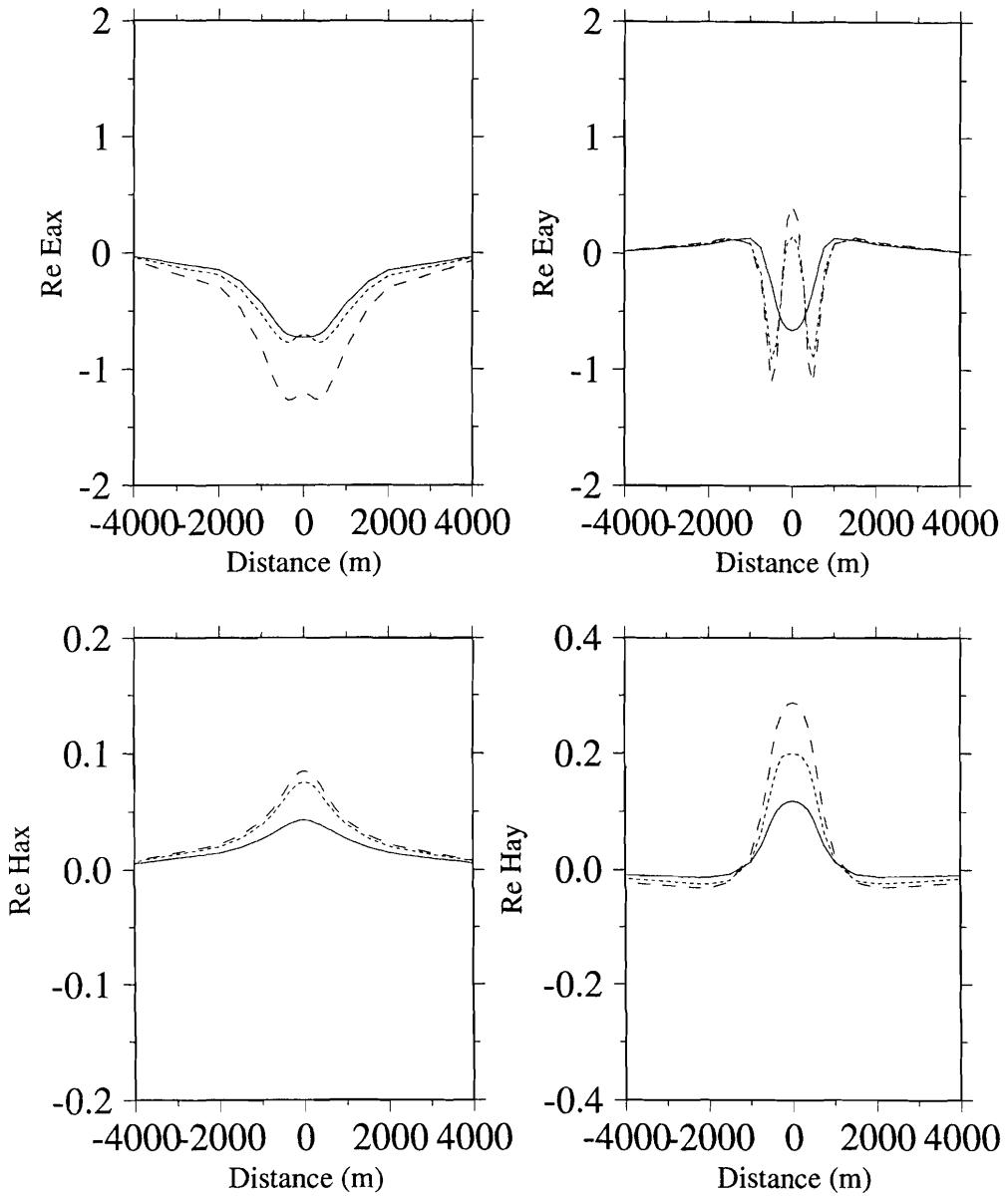
**Figure 8.** Numerical comparison of full IE solution (solid line), the modified Born approximations of the seventh order (dashed line), and the ninth order (dotted line) computed for model 3 (Figure 6) at frequency 1 Hz. Calculations are done for receivers located along the Y axes on the surface.
