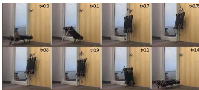
Fig. 1. Sequence of images depicting the dynamic door opening method for Minitaur in a door environment for which it is quasi-statically mismatched.
